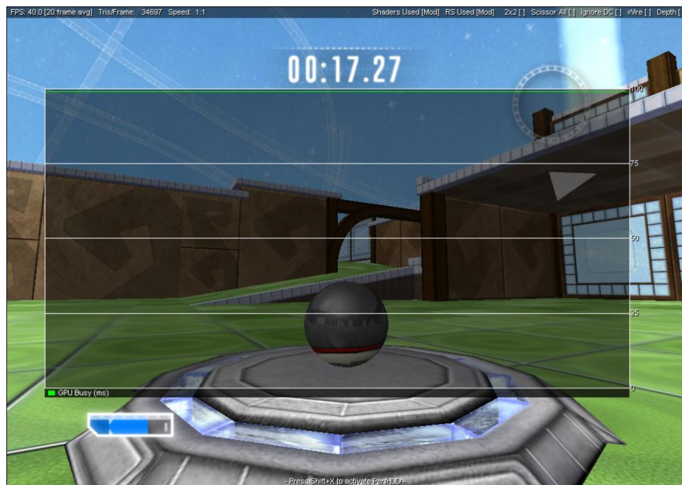
Figure 4. GPU Utilization is near 100%. This data is represented by the green line that is near the top of the chart.
