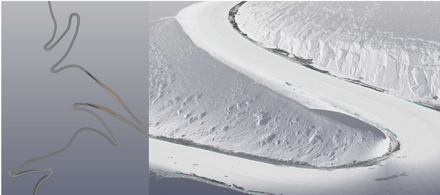
Vectorized 3D Road data and high-definition laser scanner point cloud
