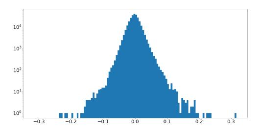
weight of layer3.4.conv3 in resnet50(torchvision), fine tuned for 4bit
