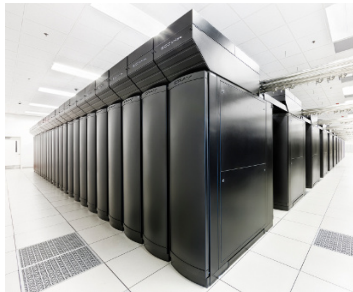
NCSA Blue Waters Hybrid Cray XE6 / XK7 22,640 XE6 dual-Opteron CPU nodes 4,224 XK7 nodes w/ Tesla K20X GPUs
