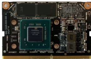
JETSON NANO 5 - 10W 0.5 TFLOPS (FP16) 45mm x 70mm $129 AVAILABLE IN Q2
