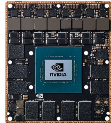
JETSON AGX XAVIER 10 - 30W 10 TFLOPS (FP16) | 32 TOPS (INT8) 100mm x 87mm $1099
