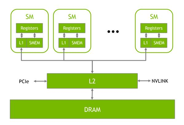
Up to 80 Streaming Multiprocessors 256KB register file per SM
