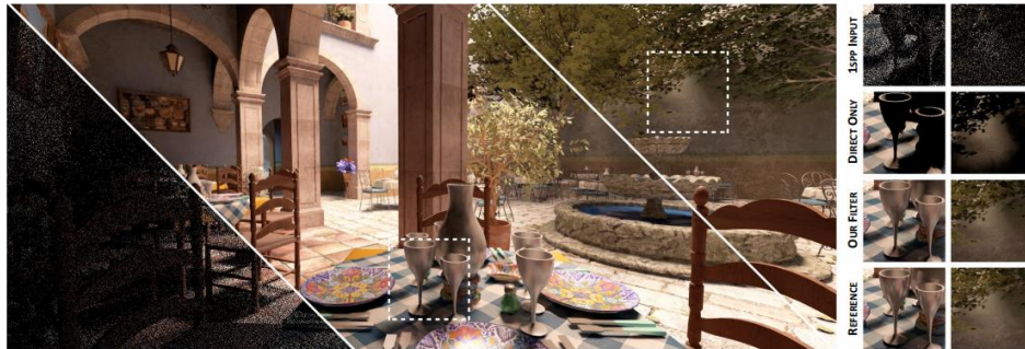
Figure 1: Our filter takes (left) 1 sample per pixel path-traced input and (center) reconstructs a temporally stable 1920×1080 image in just 10 ms. Compare to (right) a 2048 samples per pixel path-traced reference. Insets compare our input, our filtered results, and a reference on two regions, and show the impact filtered global illumination has over just direct illumination. Given the noisy input, notice the similarity to the reference for glossy reflections, global illumination, and direct soft shadows.
