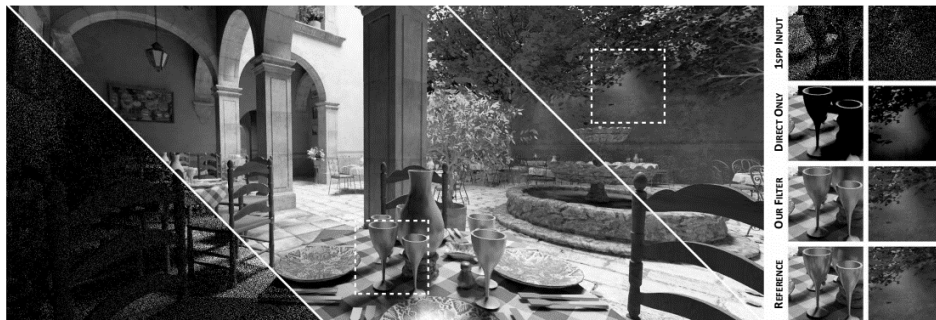
Figure 1: Our filter takes (left) 1 sample per pixel path-traced input and (center) reconstructs a temporally stable 1920 \times 1080 image in just 10 ms. Compare to (right) a 2048 samples per pixel path-traced reference. Insets compare our input, our filtered results, and a reference on two regions, and show the impact filtered global illumination has over just direct illumination. Given the noisy input, notice the similarity to the reference for glossy reflections, global illumination, and direct soft shadows.
