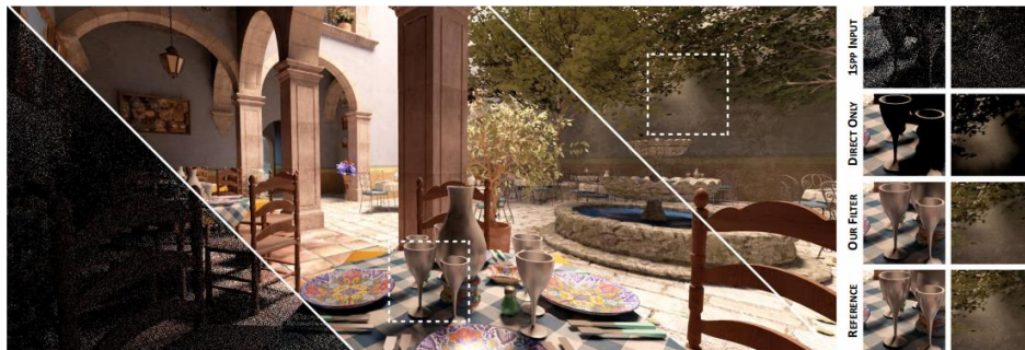
Figure 1: Our filter takes (left) 1 sample per pixel path-traced input and (center) reconstructs a temporally stable 1920×1080 image in just 10 ms. Compare to (right) a 2048 samples per pixel path-traced reference. Insets compare our input, our filtered results, and a reference on two regions, and show the impact filtered global illumination has over just direct illumination. Given the noisy input, notice the similarity to the reference for glossy reflections, global illumination, and direct soft shadows.
