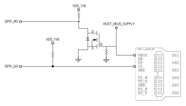
Figure 2. Example of general design for VBUS\_DETECT pin
