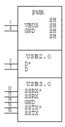
The D+/D- signal pins connect to UTMI pads. The SSTX/SSRX signal pins connect to UPHY and are handled by a single UPHY lane. As UPHY lanes are shared between PCIE, SATA, UFS, and XUSB, UPHY lanes must be assigned according to the custom carrier board's requirements.
