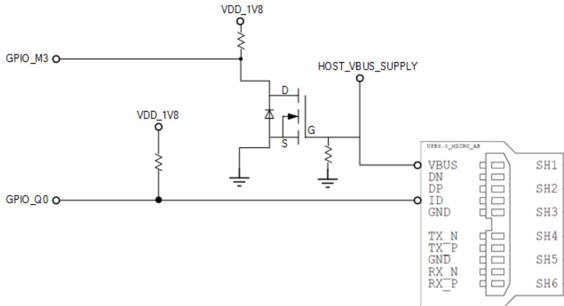
Figure 2. Example of general design for VBUS\_DETECT pin
