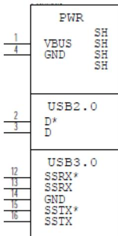
The D+/D- signal pins connect to UTMI pads. The SSTX/SSRX signal pins connect to UPHY and are handled by a single UPHY lane. As UPHY lanes are shared between PCIE, SATA, UFS, and XUSB, UPHY lanes must be assigned according to the custom carrier board's requirements.
