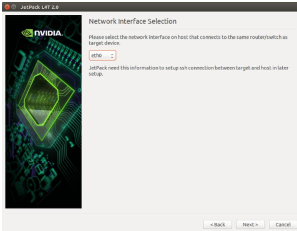
11. If you selected the **Device get IP assigned by DHCP server on host and access Internet via host machine** layout, you must select which interface to use for Internet access and which to use for the target interface.
