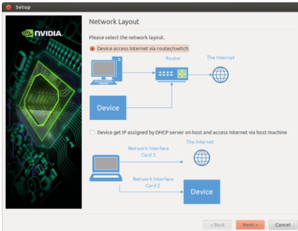
10. If you selected the **Device access Internet via router/switch** layout, you must select which interface to use for Internet access.
