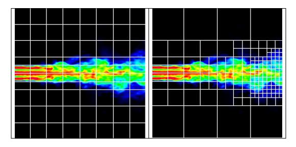
With CUDA Dynamic Parallelism, the grid resolution can be dynamically adapted at run time based on the simulation data. Starting with a coarse grid, the simulation can "zoom in" on areas of interest and avoid unnecessary calculation in areas with little change. While this could be done using CPU launched kernels, it is more efficient for the GPU to refine the grid directly by analyzing and launching additional work as needed.
