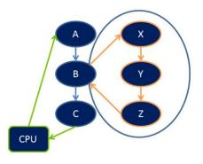
able to begin execution until kernel Z has completed, because kernels X, Y and Z are seen as part of kernel B.
