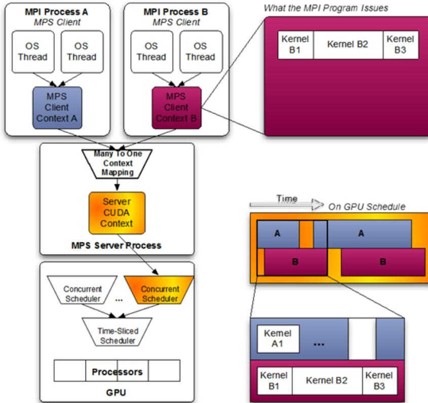
When using MPS, the server manages the hardware resources associated with a single CUDA context. The CUDA contexts belonging to MPS clients funnel their work through the MPS server. This allows the client CUDA contexts to bypass the hardware limitations associated with time sliced scheduling, and permit their CUDA kernels execute simultaneously.
