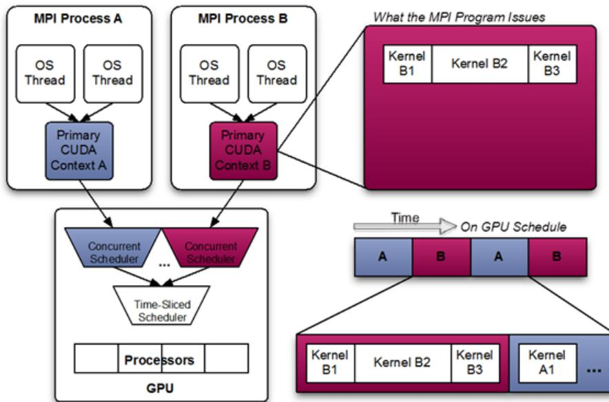
This diagram shows a likely schedule of CUDA kernels when running an MPI application consisting of multiple OS processes without MPS. Note that while the CUDA kernels from within each MPI process may be scheduled concurrently, each MPI process is assigned a serially scheduled time-slice on the whole GPU.
