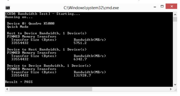
The device name (second line) and the bandwidth numbers vary from system to system. The important items are the second line, which confirms a CUDA device was found, and the second-to-last line, which confirms that all necessary tests passed.
