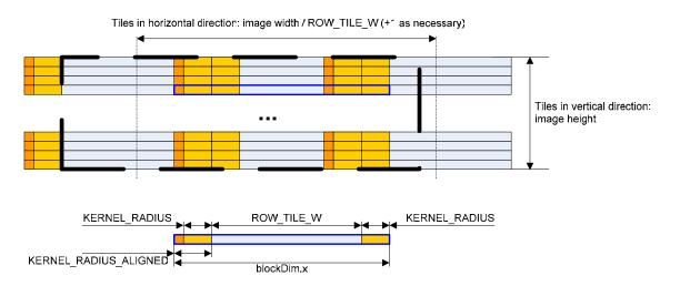
Figure 10: Layout of the thread block grid for the row filtering pass.
