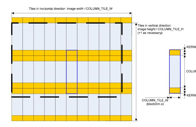
Figure 12: Layout of the thread block grid for the column filtering pass.
