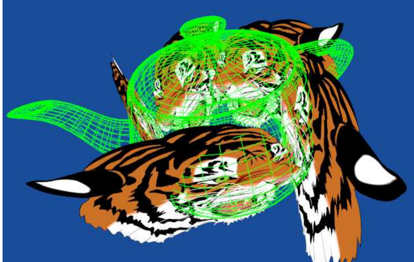
Figure 5: An enlarged green wireframe teapot protruding through an arrangement of five tigers to show how depth testing is correct even for complicated wireframe geometry.
