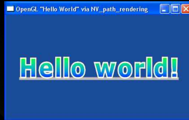
pr_hello_world: kerned, underlined, stroked, and linear gradient filled text
