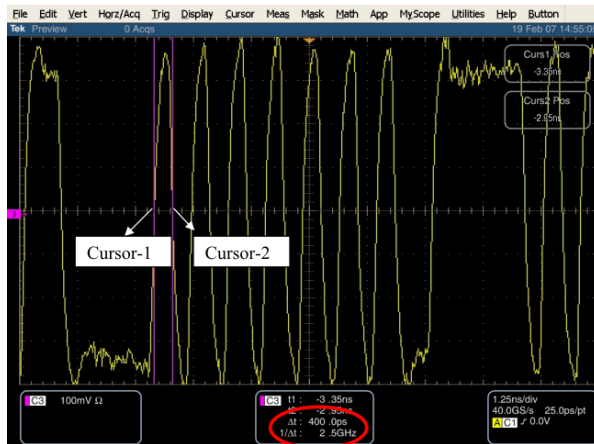
Figure 8. Gen1 Data Signal at 2.5 GT/s Showing User Interface = 400 ps
