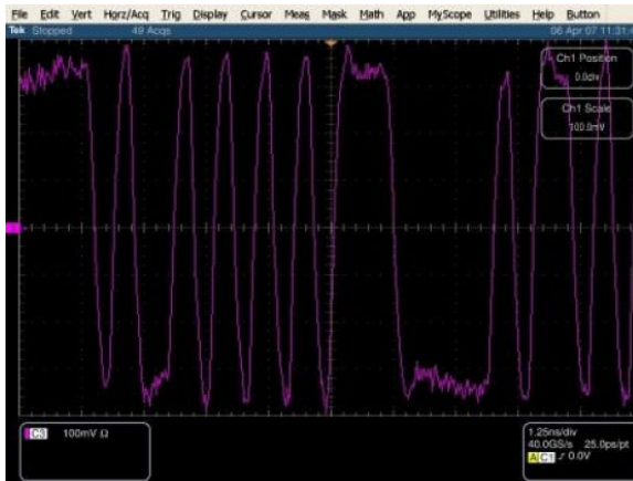
Figure 7. Differential Data Signal Waveform
