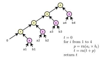
Figure 2: The serial method uses a simple loop with separate multiplies and adds to compute the dot product of the vectors. The final result can be represented as  $((((a_1 \times b_1) + (a_2 \times b_2)) + (a_3 \times b_3)) + (a_4 \times b_4))$ .
