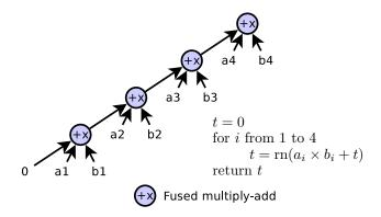
Figure 3: The FMA method uses a simple loop with fused multiply-adds to compute the dot product of the vectors. The final result can be represented as  $a_4 \times b_4 + (a_3 \times b_3 + (a_2 \times b_2 + (a_1 \times b_1 + 0)))$ .
