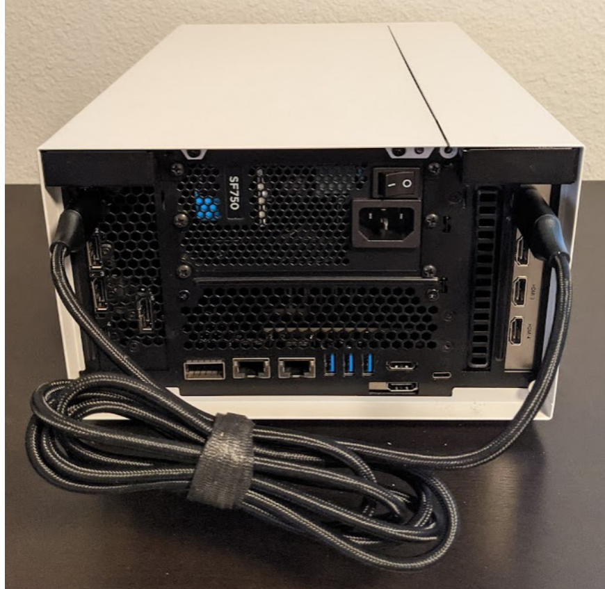
Fig. 37.2: DP-to-HDMI Cable Between GPU and AJA KONA HDMI Capture Card (Channel 1)
