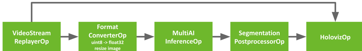
Fig. 8.6: The BYOM inference workflow
