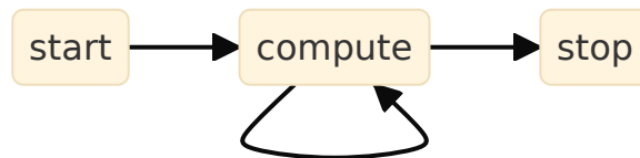
Fig. 9.4: The sequence of method calls in the lifecycle of a Holoscan Operator
