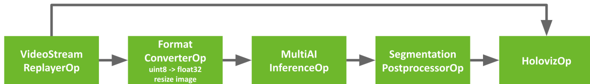
Fig. 7.5: The BYOM inference workflow
