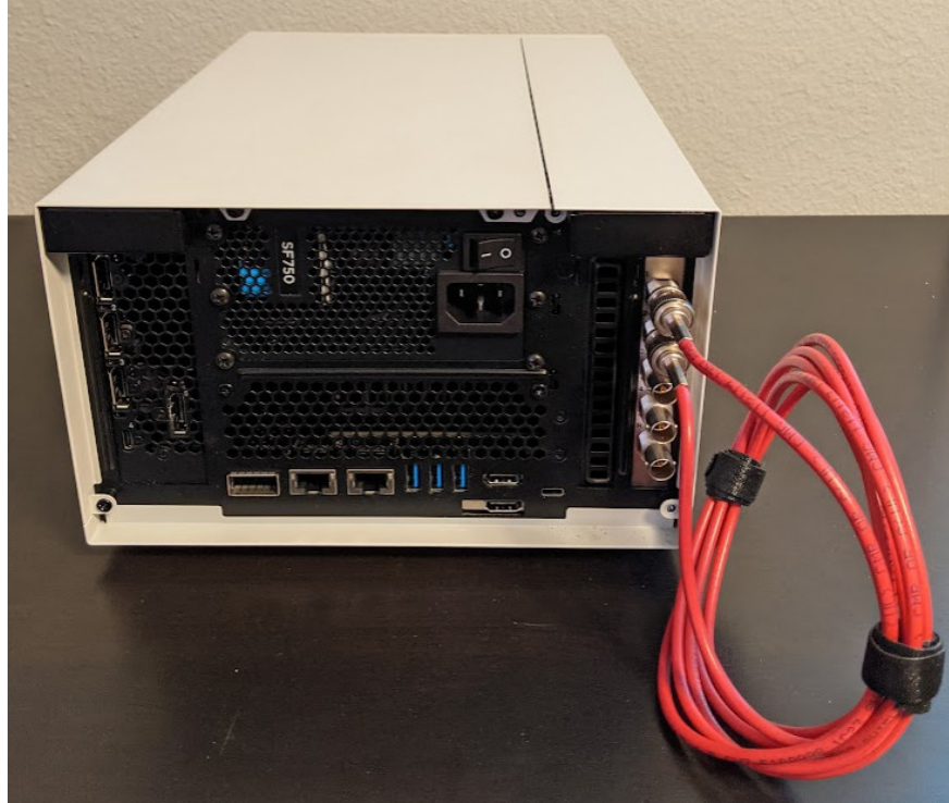
Fig. 19.3: SDI Cable Between Channel 1 and 2 of a Single AJA Corvid 44 Capture Card
