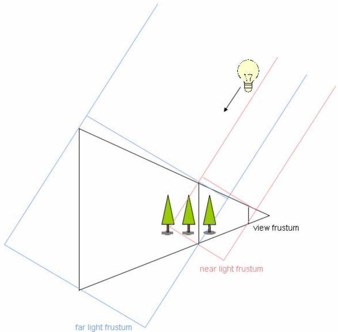
**Figure 1-1.** The right-most tree is captured in the near shadow-map and the other two are in the left. As seen from a viewer on the side, the left shadows are blocky, however, the camera would perceive all 3 shadows with approximately the same aliasing.
