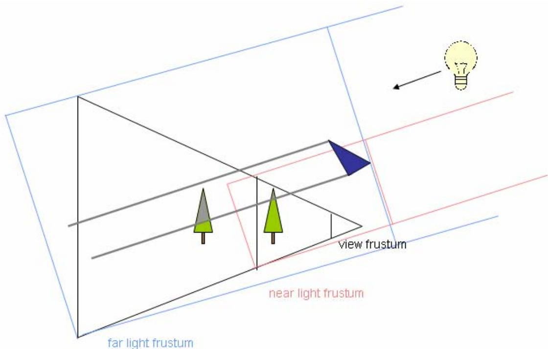
**Figure 2-4.** A triangle casting a shadow in multiple depth maps
