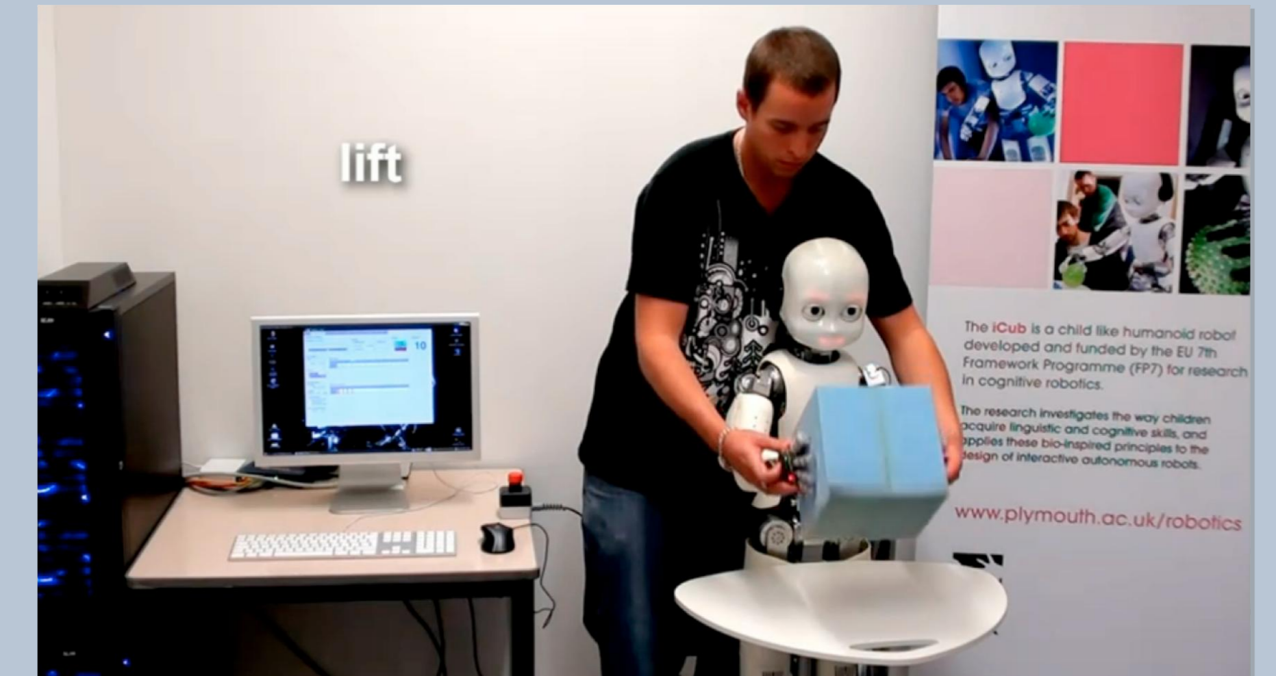
The Sequence Recorder module of Aquila was used to record these sensorimotor patterns while the experimenter was guiding the robot by holding its arms and performing the actions.
