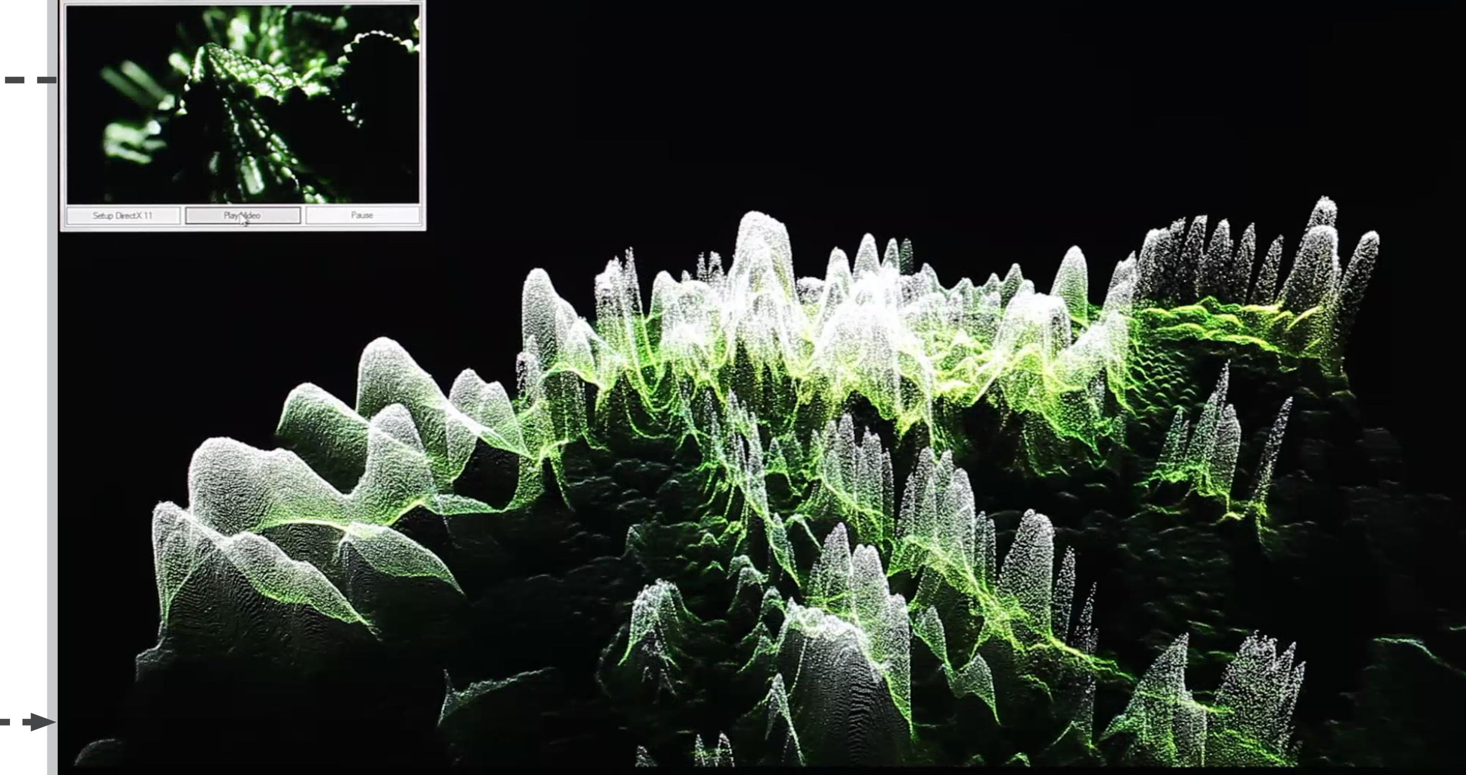
By mapping a video source into 3D space, each pixel can be displayed highly differentiated. This approach could be utilized for checking video quality on lower pixel level like on a realtime video waveform monitor. For digital content creation this experiment may provide new possibilities for particle-based visual effects that allow to dissolve a video source into a highly dynamic 3D point cloud.
