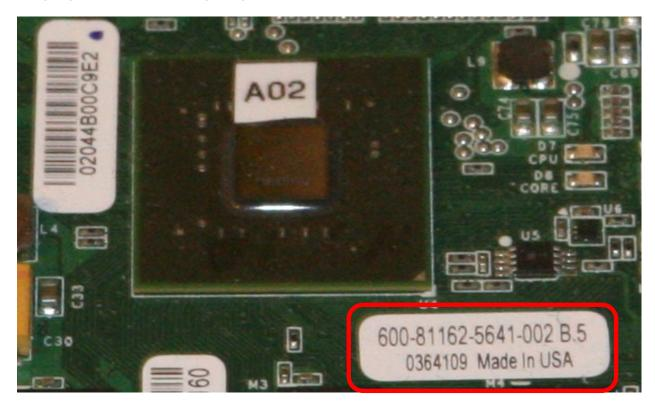
The serial number can be decoded as follows:
