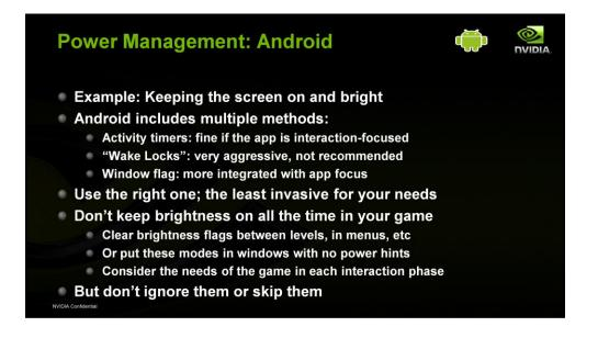
A quick look at power management in Android by looking at the 600 milliwatt gorrilla: screen and backlight. Android has aggressive power management as you'd expect, and the screen and backlight are core targets for power management
