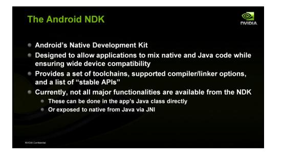
Google provides the Android NDK, or native development kit. This is a set of toolchains, makefiles, and headers and libs that expose a set of "stable" APIs. The concept of "stable" here is not runtime stability, as much as API and ABI stability across Android versions and hardware. This does mean that not all Android or Linux functionalities are available via the NDK. So what did and didn't make the current cut?
