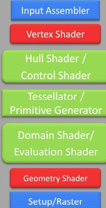
The tessellation engine has three stages, two of them are programmable (the hull and domain shader) and one of them is fixed function (the tessellator).
