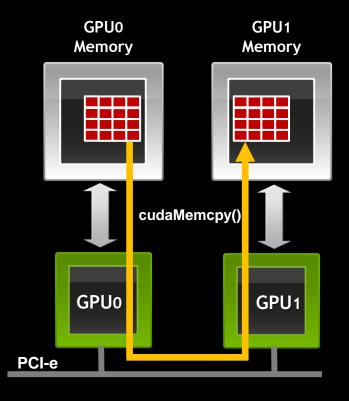
Eliminates system memory allocation & copy overhead More convenient multi-GPU programming
