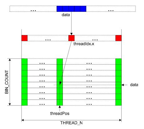
Figure 1. s\_Hist[] array layout for histogram64.
