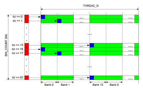
Figure 2. Shifting start accumulation positions (blue) in order to avoid bank conflicts during the reduction stage in histogram64.
