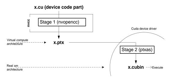
By specifying a virtual code architecture instead of a 'real' GPU, nvcc postpones the second compilation stage until application runtime, at which the target GPU is exactly known. For instance, the command below allows generation of exactly matching GPU binary code, when the application is launched on an*sm\_10*, an *sm\_13*, and even a later architecture
