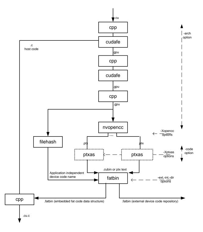
Figure 2: CUDA compilation from .cu to .cu.cpp.ii
