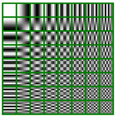
Figure 3. 2D basis functions for N = 8.
