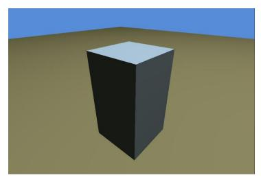
The next step is to add simple shading to the objects in the scene. To do this, we just rewrite the closest hit program to do a lighting calculation at each hit point.
