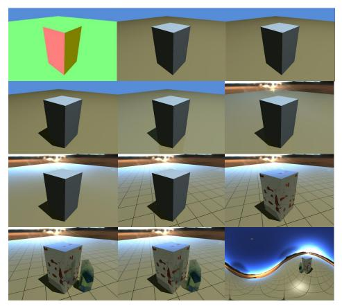
The OptiX SDK provides a source code sample, *tutorial*, that demonstrates how to implement several basic ray tracing effects, from trivially simple to moderately complex. The sample consists of eleven stages, each stage adding a new effect. In this section, we discuss each of these stages and show programs for both shading and intersection.
