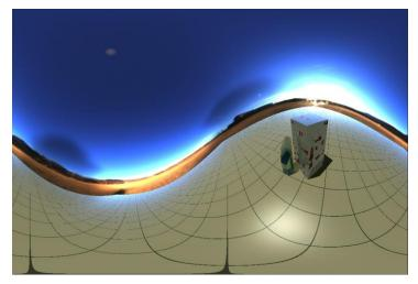
Our final tutorial demonstrates the flexibility of OptiX (and ray tracing in general) by modifying the pinhole camera ray generation program from the very first example. This new camera shoots rays in a spherical distribution, resulting in an image that can then be used as an environment map in another program, or even as a background image in tutorial step 5.
