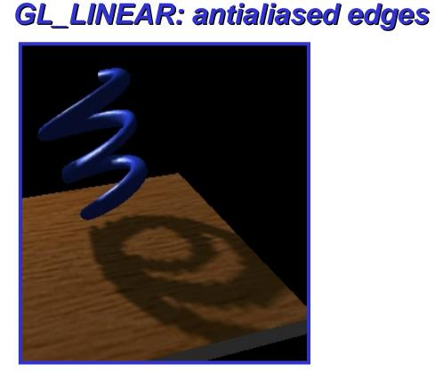
Low shadow map resolution used to heightens filtering artifacts
