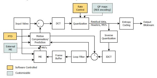
Figure 1. NVENC hardware block diagram
