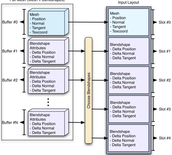
The number of blend shapes we can append depends on how they fit in the 16 available attributes. It could be possible to add more blend shapes in additional slots if we compressed the data (normalized vectors packed in 32bits or using fewer
