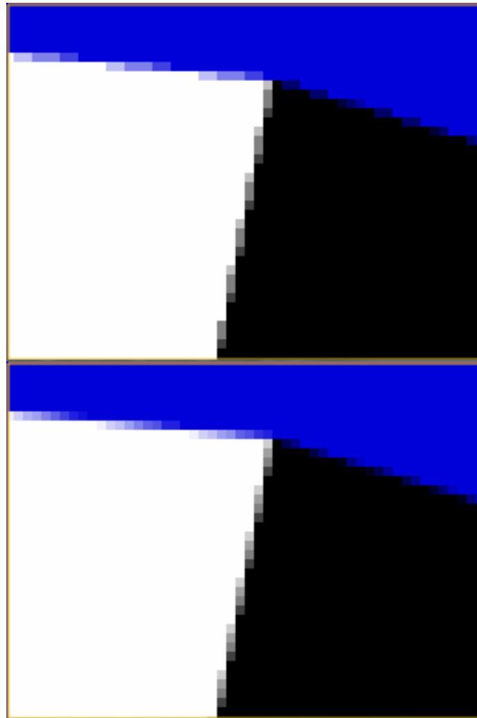
Figure 2. CSAA – 4x vs. 16x
