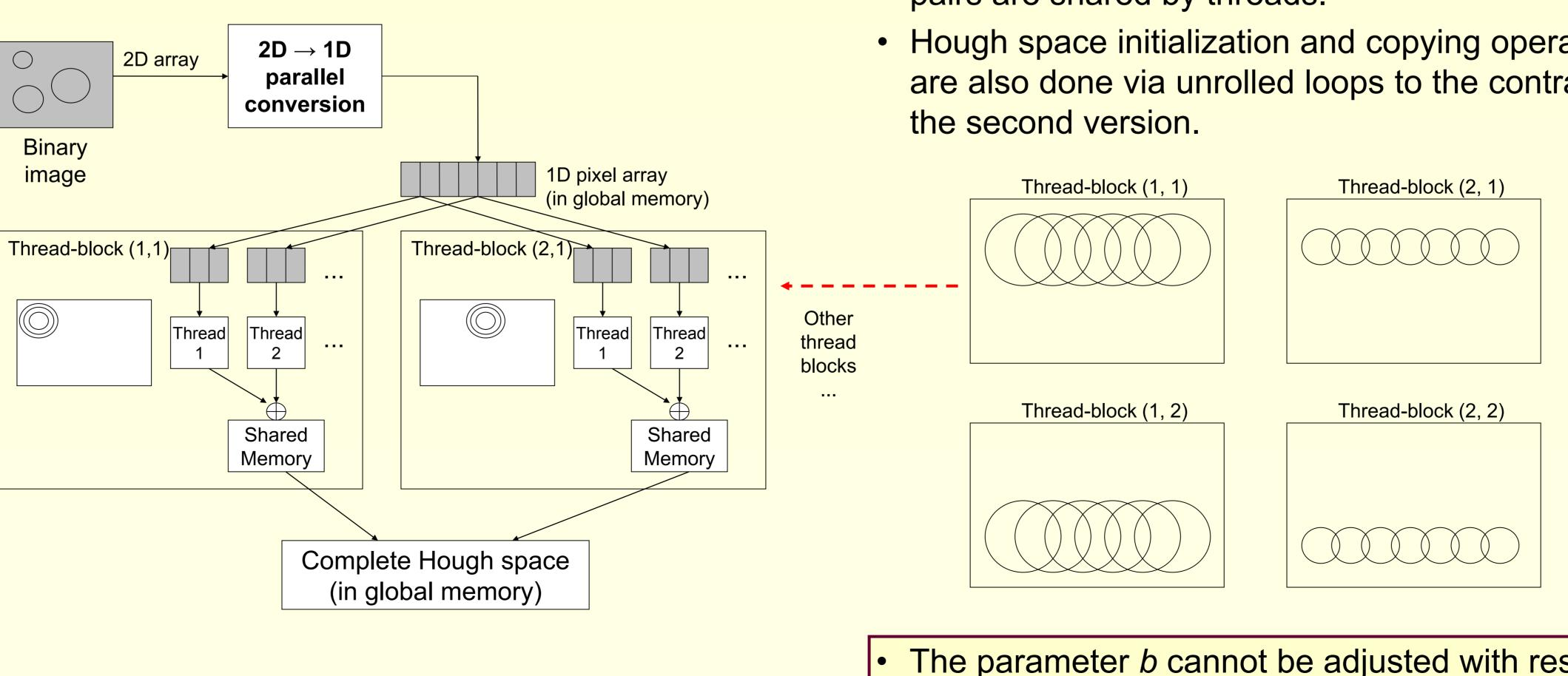
Parallelization of Hough Transform for Circles using CUDA
