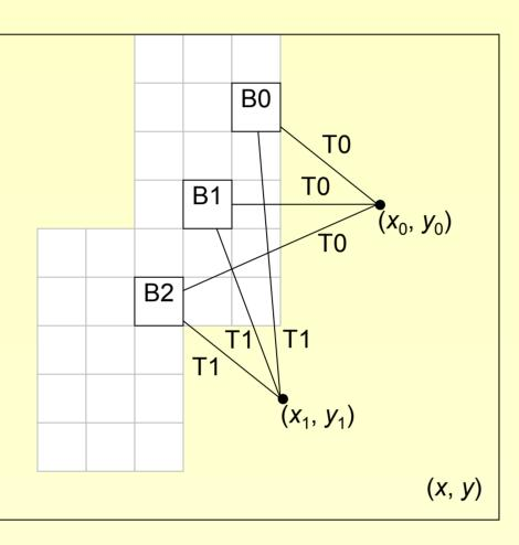
Thread-blocks {B0, B1, B2 ...} sharing circle centers (a, b) and threads  $\{T0, T1 \dots\}$ sharing the points  $\{(x_0, y_0),$  $(x_1, y_1) \dots$  in the image.
