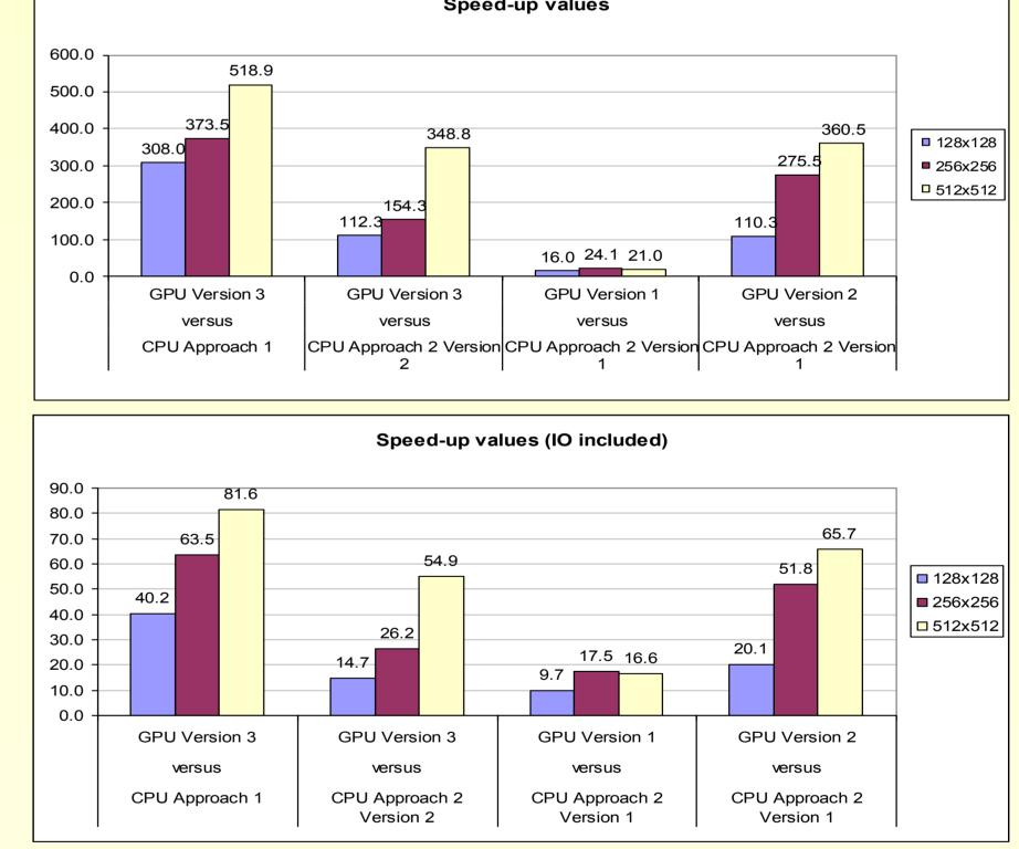
Speedup increases with image size. • Up to ~360 times speedup for GPU Version 2 and up to ~350 times speedup for GPU Version 3. Speedups degrade significantly when IO transfer
